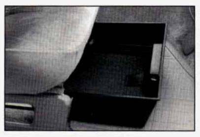
If you have an optional sliding tray storage compartment, it is under the front passenger seat. To open the compartment, move the latch in the top handle and pull the tray forward.
